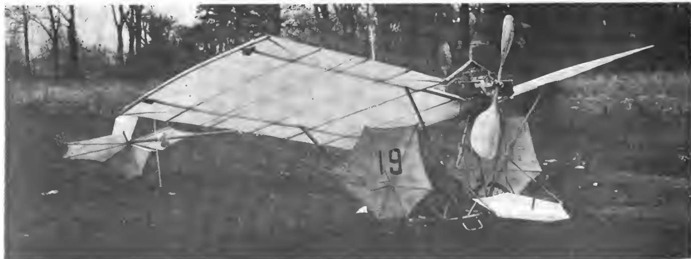
"THE BUTTERFLY," NINETEENTH AEROPLANE CONSTRUCTED BY SANTOS-DUMONT SMALLER AND LIGHTER THAN PREDECESSORS.
